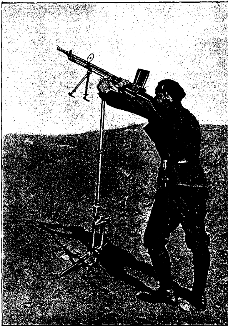
ZB 30 mounted on tripod adjusted for anti-aircraft firing
